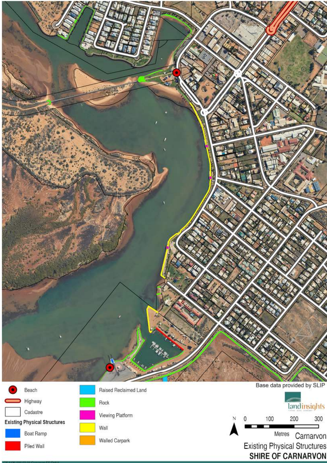
Map 3.10 – Existing physical structures – Carnarvon (detail)
