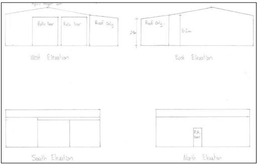
Figure 2: Elevations of shed
