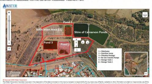
Map 3 below identifies the location of the new infrastructure and operational assets to replace the old infrastructure used for the filtration and chlorination of wastewater from the Carnarvon Wastewater Treatment Plant:
