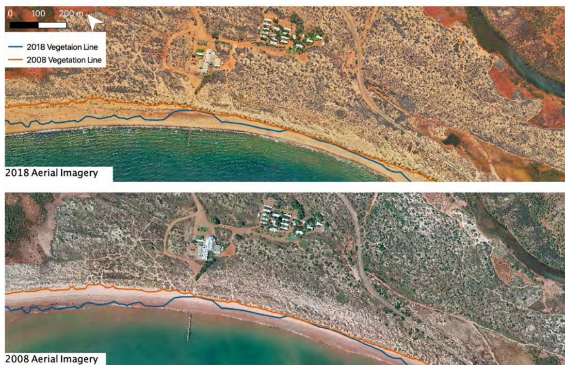
Figure 7: Coastline Movements from 2008 to 2018 show an historic trend (S2) of stability or accretion adjacent to the development, rather than the erosion trend identified in GEMS 2009
