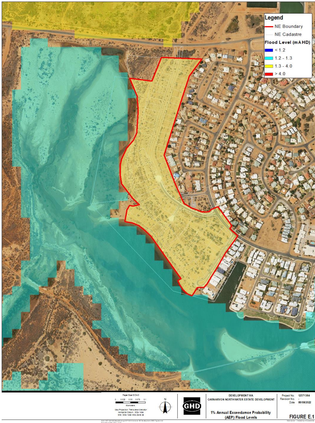
Figure E.1 Northwater Estate 1% AEP flood levels and extents
