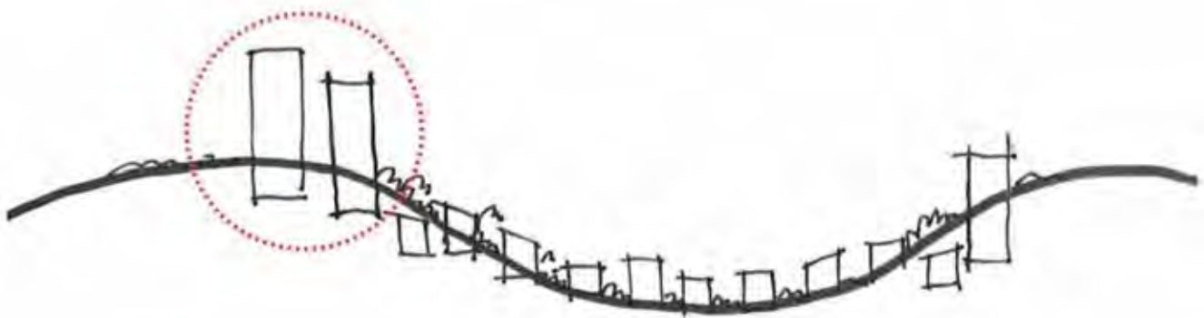
Figure 4: Model proposed development to assess “skylining” of development. Reconsider development that it out of scale in relation to surrounding built form and landscape features
