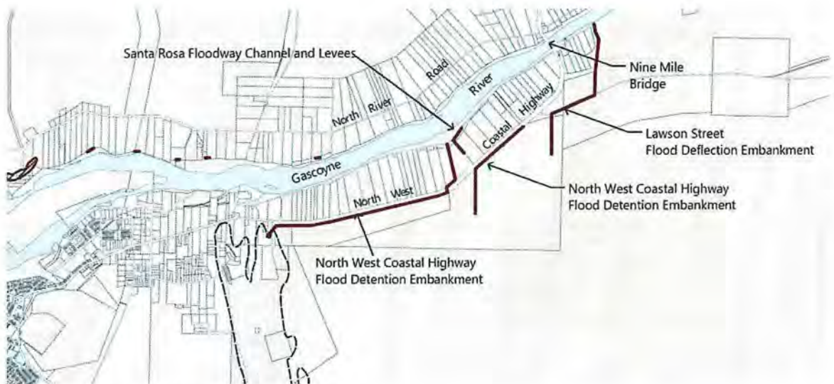
Figure 31. Structural measures to address flooding
