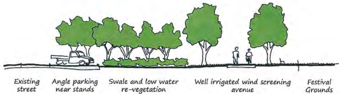
Figure 65. Possible design to address wide road reserve on Gascoyne Road (showing half reserve).
