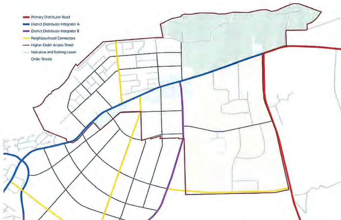
Figure 57. Structure Plan Movement Hierarchy (Includes 50 year+ Indicative Long Term Vision for Carnarvon Airport Precinct)
